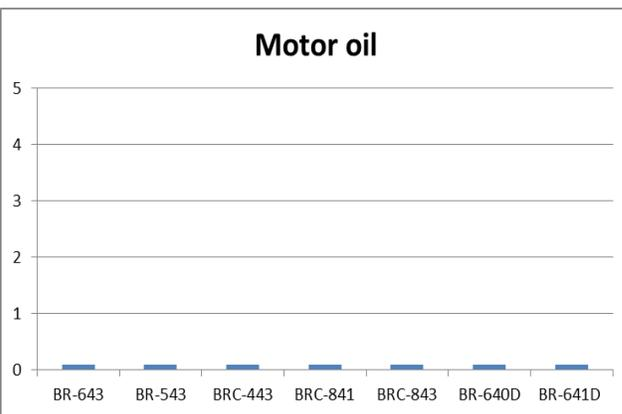
Figure 12. Chemical Resistance Against Motor Oil
