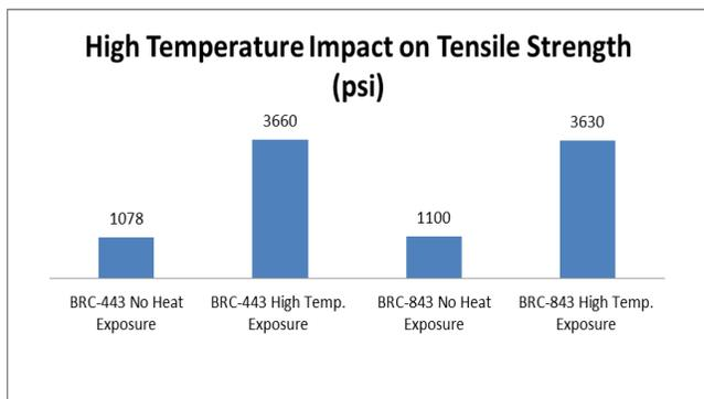
Figure 14. High Temperature Impact on Tensile Strength (psi)
