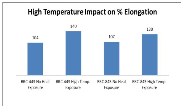
Figure 13. High Temperature Impact on Elongation (%)
